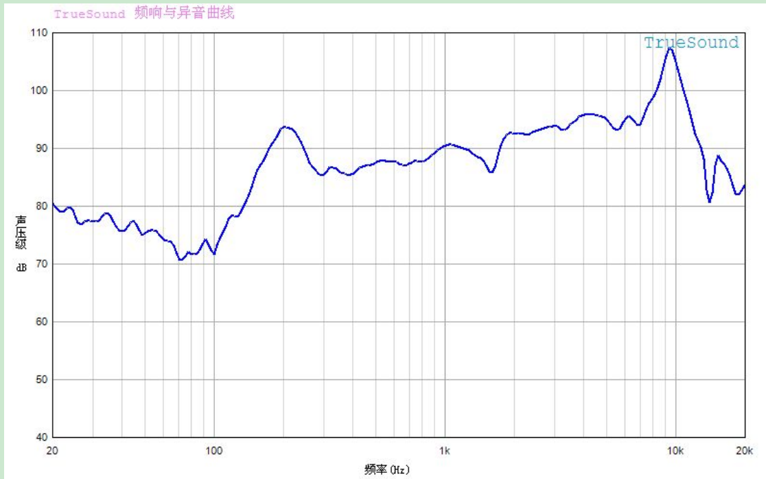
Fig.2 Frequency response mask & typical frequency response curve (speaker mode)
